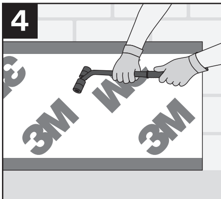
4 Roll the membrane with a rubber roller to ensure a tight bond to the wall and overlaps.
